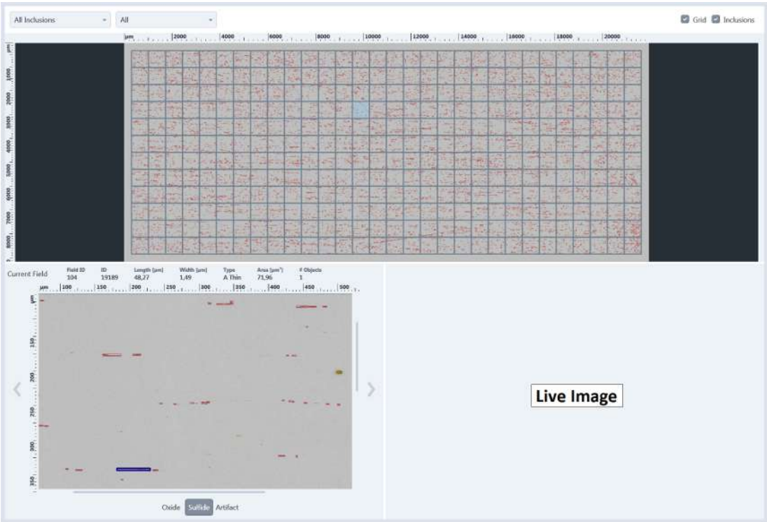
Fig. 51: Example: NMI Analysis Field based inspection with live navigation on the specimen to inspect standard specific inclusion types.
