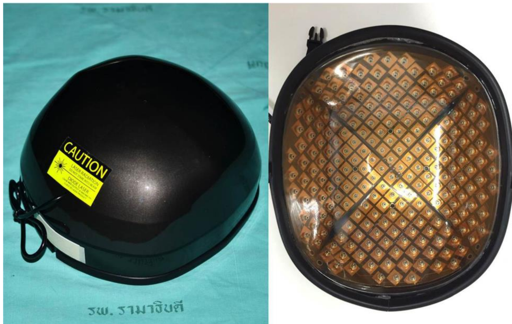
Figure 1. RAMACAP, a helmet-type portable LLLT device containing 224 red diode laser bulbs (660 nm)
